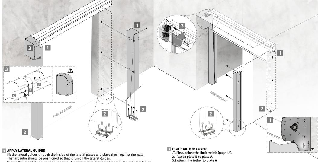
Secure the lateral guides to the support plates with screws, tightening them in the nuts located on the lateral guides.
